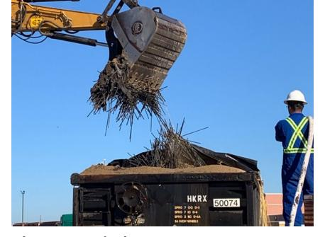
The Zirc Rods were dispersed throughout the gondola in no certain arrangement and were observed and photographed of various lengths. Some of the Zirc Rods were banded tighter and other looked to be used, flattened raggedly cut and ready for disposal. Because of the various degrees of the conditions of these rods, the Zirc Rod entry on the shipping paper became a question. At that point FRA began inquiring with the shipper and metallurgy experts for more details about the Zirc Rod entry.
